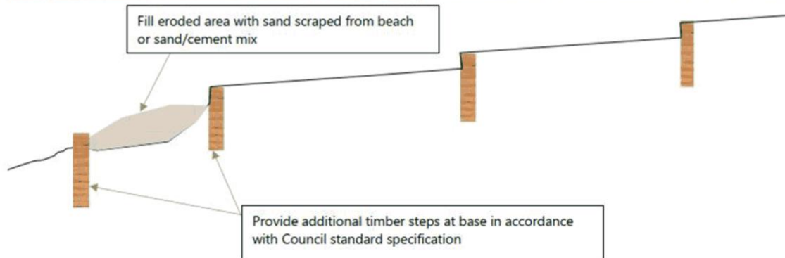
Figure 5-4 – Recommended treatment for erosion at base of access, where gradient is low - moderate (see examples above)
